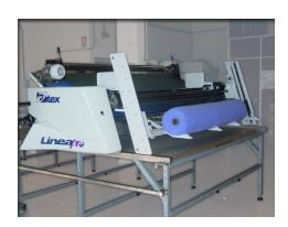
Loader for Linea Pro spreading machine. It loads from the floor to the cradle. Maximum roll weight: 100Kg.
