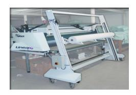
Loader for Goliat 300 folding cradle spreading machine. It loads and unloads from the floor to the cradle and is specially design for jeans or heavy fabric. Maximum roll weight: 300Kg.
