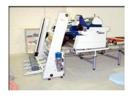
Carleans Loader for Goliat 300 spreading machine special for jean fabric rolls. It loads and unloads with a support bar from the floor to the cradle. Maximum roll weight: 300Kg.
