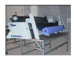
Cargo 1 Loader attached to the Linea Plus spreading machine. It has the same characteristics of Cargo 80.
