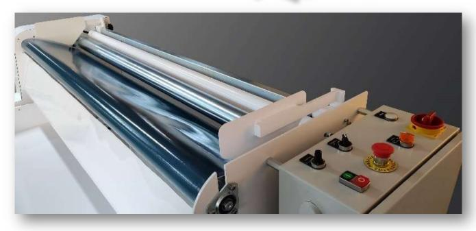
Our Autex Desroll machine allows you to unroll the fabric rolls easily so that they can relax and thus avoid shrinkage during spreading.
