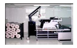
Cargo Loader for Tecno spreading machine. It loads from the floor to the cradle. Maximum roll weight: 100Kg.
