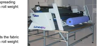
**Cargo** Loader attached to the Linea Pro spreading machine. Loads the fabric rolls from the table to the cradle or to the support bar system. Maximum roll weight: 100Kg.
